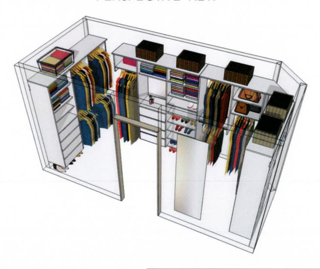
All Shelves are to be fixed and not adjustable. All Joinery units will be secured to the Wall. Units will have NO backs unless specified, so you will see the wall colour behind
